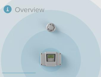
The Wi-Fyre Wireless Optical Detector consists of a ProFyre optical smoke detector head combined with a Wi-Fyre wireless base. The Wi-Fyre Optical Smoke Detector uses a pulsing IR LED & photodiode to detect IR scatter caused by smoke entering the chamber.
